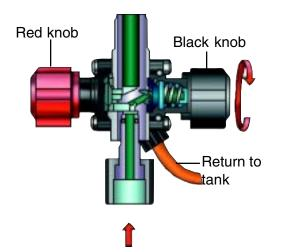
"The multifunction valve screws directly onto the discharge valve of the metering pump.
