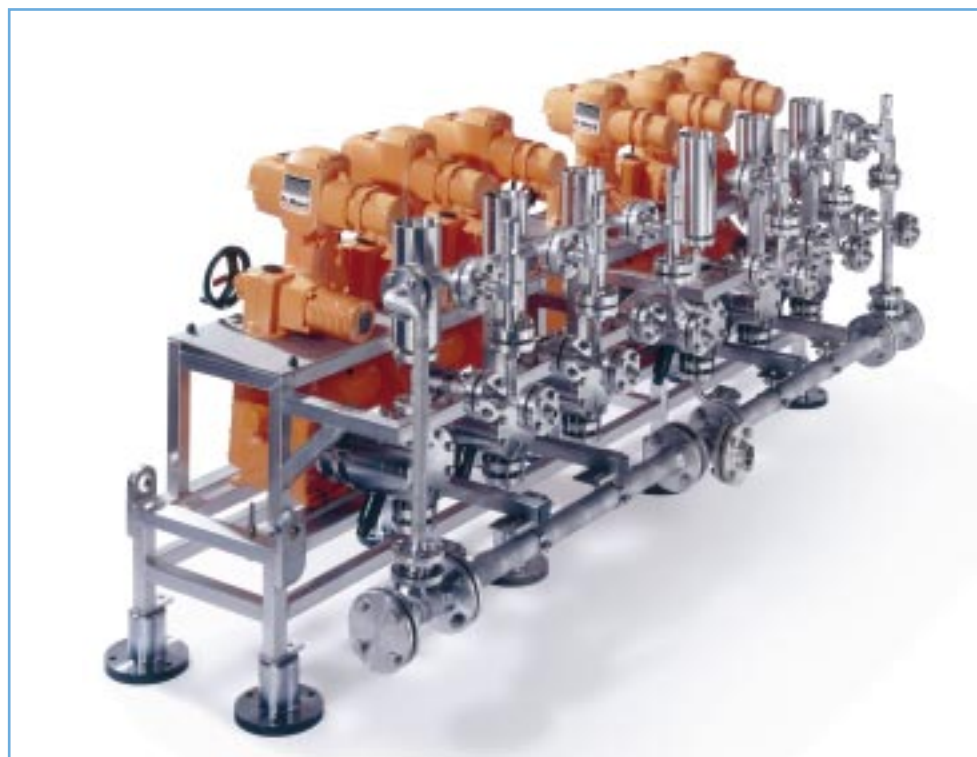
Injection Skid with 6 headed pump, 6 x 79 gph at 588 psig (300 l/h at 40 bar)
