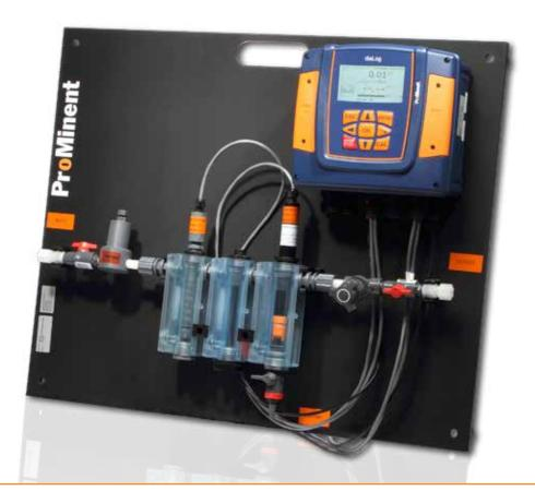
**ProMinent® Packaged Analyzers** provide precise monitoring or control of chlorine for potable and wastewater applications. These engineered systems utilize the latest amperometric sensor technology resulting in a "reagent free" on-line analysis with no colorometric concerns or reagents.
