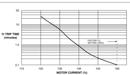
FIGURE 23 - I't TRIP TIME vs MOTOR CURRENT
