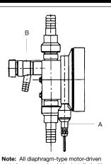
Note: All diaphragm-type motor-driven metering pumps should be installed with a pressure relief valve on the discharge line; however, with the Sigma HM pump, integral pressure relief valve is optional. See the High-Flow Accessories section of the catalog for pressure relief valves if integrated pressure relief is not provided.
