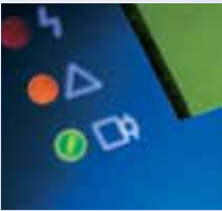
LED status indicators warn of operating faults
