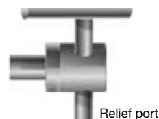
Backpressure valve on tee for pressure relief
