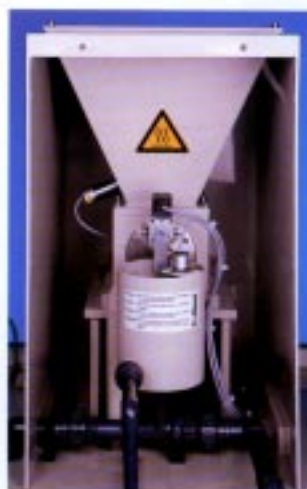
Dry Feeder with wetting cone
