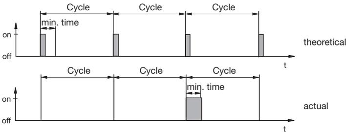
The DULCOMETER® D1C does not switch for a certain number of cycles until the sum of the theoretical switching times exceeds the “min. time”. Then the DULCOMETER® D1C switches for the duration of this total time.
