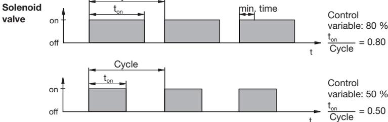
The switching time of the DULCOMETER® D1C (solenoid valve) depends on the actuating variable and the “min. time” (smallest permitted operating factor of the connected device). The actuating variable determines the ratio  $t_{on}/cycle$  and thus the switching times (see fig. above).
