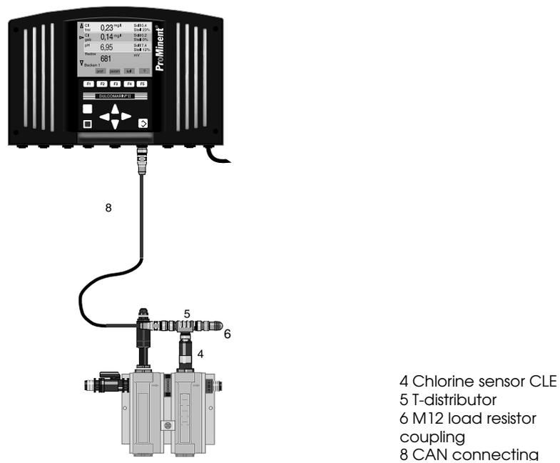
Abb. 3: CAN connection of an individual chlorine sensor
