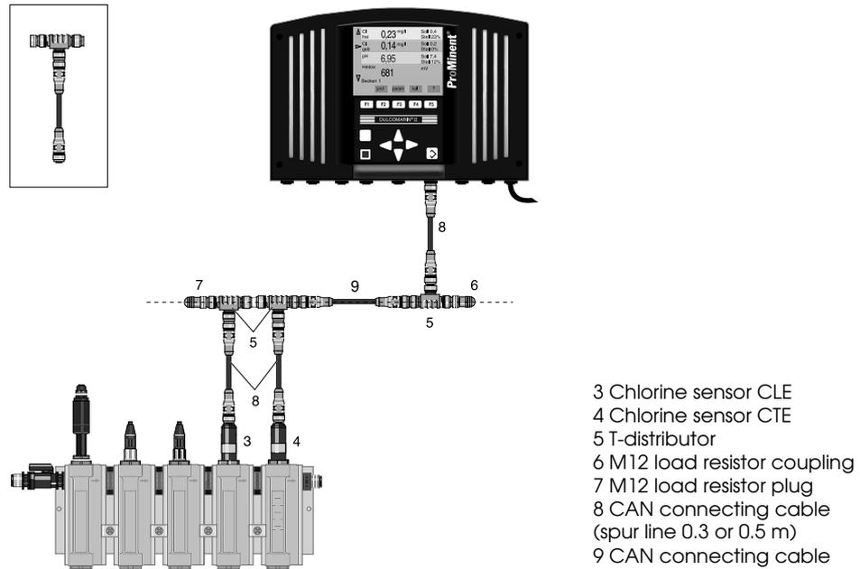
Abb. 2: CAN connection of two (more) chlorine sensors
